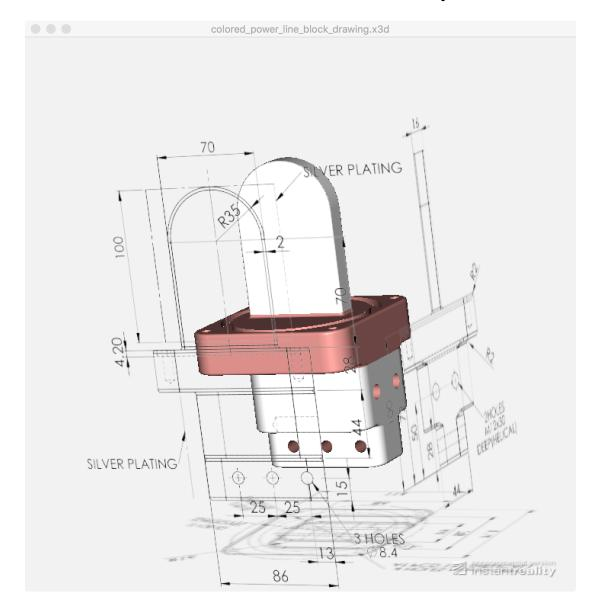
Rendered in X3D Source was STEP solid model and PNG images for 2D drawings.
