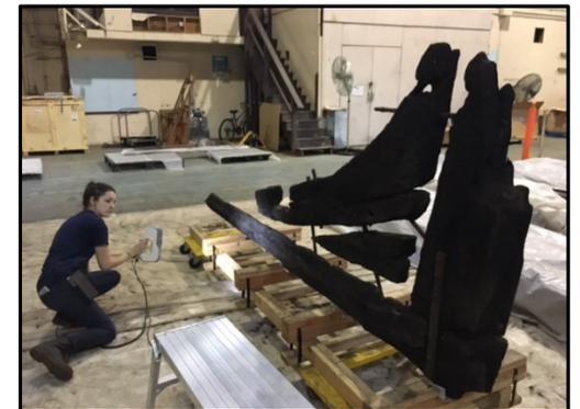
Artec Eva Scanner and Processing Software
