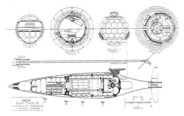
Fig. 2. Schematic design of Seaglider. The bottom shows a side view with the wing shape provided above for reference. The antenna mast is shown separately above the fairing and pressure hull. Four cross-sectional views at an expanded scale are shown at the top of the figure.
