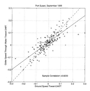
Fig. 9. Scatter plot of the cross-channel component of glider speed through the water over a  $\sim$  1-h dive cycle with over ground speed derived from GPS fixes. Lines indicate linear regressions of each variable upon the other.
