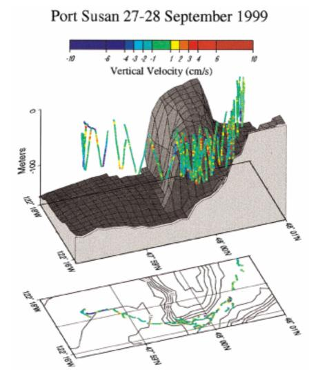
Fig. 10. Vertical velocity inferred from the difference between observed and model glider vertical motion rates in the narrow passage SE of Gedney Island connecting Port Susan (shallower, to the right as depicted) to Possession Sound (deeper, to the left).
