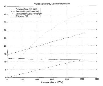
Fig. 3. Buoyancy control system pumping rate, electrical input power (current times voltage), mechanical output power (pressure times rate of volume change), and efficiency (ratio of output to input power) versus pressure.
