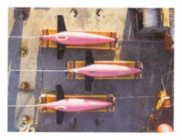
Fig. 1. Top view of three Seaglider vehicles in their handling cradles on deck. Plastic tubing is connected to the conductivity cell mounted atop the pink fairing just aft of its maximum diameter between the wings on two of the three vehicles. The white antenna masts extend aft of the fairings outside the view of this image.
