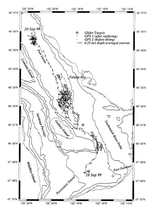
Fig. 7. Seaglider track from Port Susan to Possession Sound, September 1999. Pairs of GPS fixes are plotted between dive cycles. Arrows indicate depth averaged current inferred from the difference between actual and dead-reckoned displacements. Depth contours are in meters.
