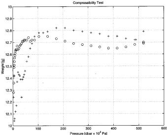
Fig. 4. Weight of Seaglider in a pressure vessel filled with de-ionized fresh water at room temperature. Symbols indicate duplicate tests. Weight changes of  $\sim 12$  g at pressures lower than 2 dbar due to air bubble compression are not shown in order that resolution at higher pressures may be higher. Differences between the tests can be attributed to load measurement errors.
